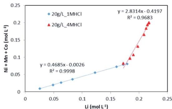
Fig. 5 Stoichiometry between the sum of Ni, Mn, Co concentration and Li concentration in leachate at  $S/L = 20 \text{ g } L^{-1}$  during NMC 811 dissolution by  $1 \text{ mol } L^{-1}$  (blue diamonds) and  $4 \text{ mol } L^{-1}$  HCl (red triangles) at  $25 \text{ }^{\circ}\text{C}$ .
