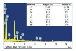
Fig. 7 Energy dispersive X-ray (EDX) image of the prepared biomagnetic membrane capsules (BMMCs). (Reproduced from Ali *et al.*<sup>24</sup> Copyright@2019, with permission from Elsevier Ltd.)
