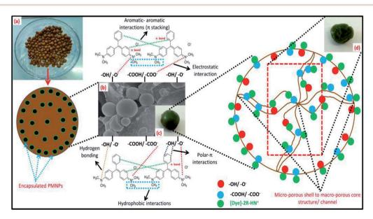
Fig. 17 Proposed adsorptive removal mechanism of cationic malachite green (MG) dye by bio-magnetic membrane capsules (BMMCs) and (a) a real pictorial representation of fabricated BMMCs, (b) SEM images of BMMCs, (c) real pictorial representation of the outer surface of the BMMCs after the sorption of cationic MG dye, and (d) a real pictorial representation of the cross-sectional/inner surface of the BMMCs after the sorption of cationic MG dye for a better understanding.
