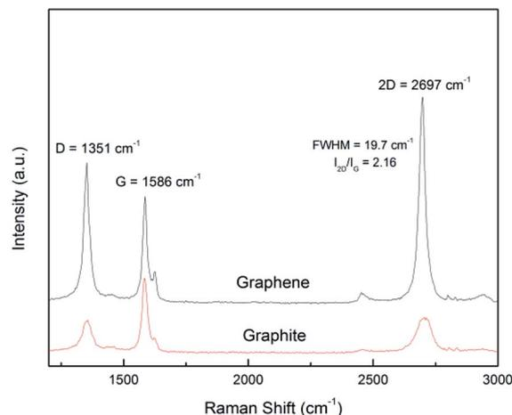
Fig. 5 Raman spectrum of graphite and exfoliated graphene.
