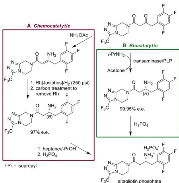
**Fig. 5** Comparison of Merck's chemocatalytic and Biocatalytic syntheses for their antidiabetic drug Sitagliptin. Reprinted with permission from AAAS.<sup>106</sup>
