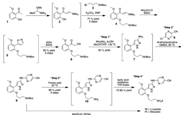
Scheme 2 Continuous manufacturing production route for prexaseritib monolactate monohydrate under cGMP conditions.<sup>112</sup> Reprinted with permission from AAAS.
