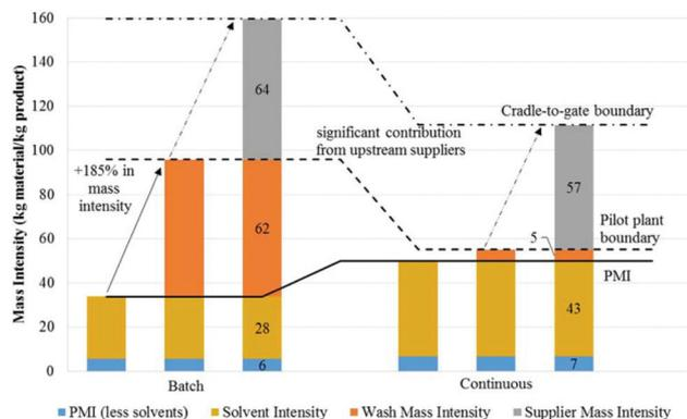
**Fig. 7** Use of Green Chemistry metrics to analyze batch & continuous processing systems. The mass intensities presented are calculated using base case values. The bolded line denotes PMI, while the dotted line denotes the mass intensity at the pilot plant level. The dash-dotted line denotes the Cradle-to-Gate (CtG) boundary and indicates the cumulative mass intensity.<sup>163</sup> Copyright (2016) American Chemical Society.
