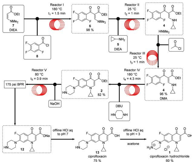
**Scheme 1** Telescoped scheme for the continuous flow production of Ciprofloxacin. Adopted and reprinted with permission from Wiley & Sons.<sup>60</sup>
