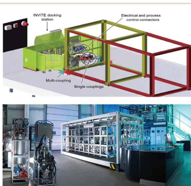
Fig. 8 Conceptual representation of the F<sup>3</sup> system (left) and manufactured version of the flexible mobile factory (right).<sup>177</sup>
