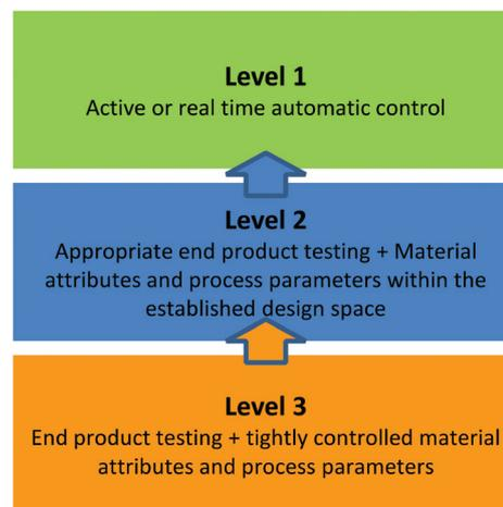
Fig. 3 Categorization of potential controls and testing levels available for control strategies in pharmaceutical manufacturing.<sup>52</sup>
