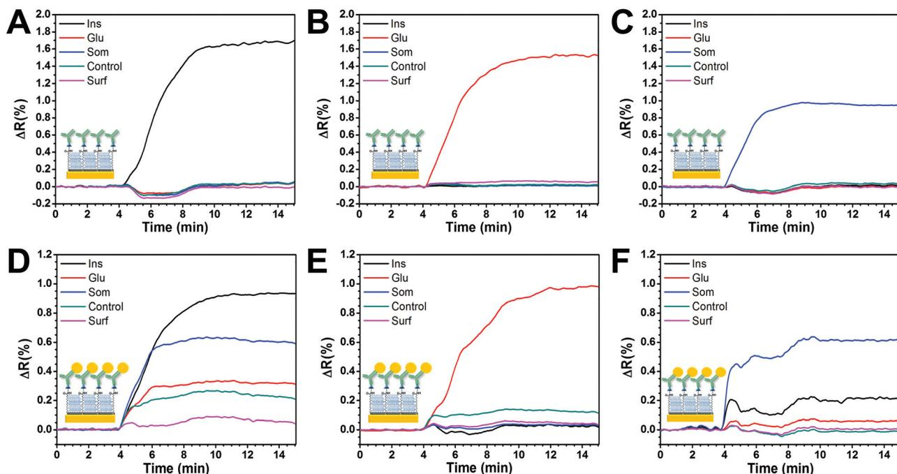
**Fig. 4** Comparison of the sensor specificity in multiplexed mode. The first row shows the specificity of the sensor without signal amplification for (A) anti-insulin, (B) anti-glucagon, and (C) anti-somatostatin. The second row shows the specificity of the sensor on the same surface with signal amplification for (D) GNP-anti-insulin, (E) GNP-anti-glucagon and (F) GNP-anti-somatostatin. Immobilized BSA ("Control") and the bare SAM surface ("Surf") were used as negative controls.
