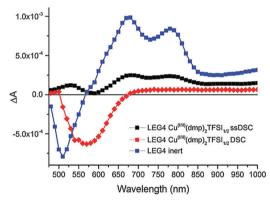
Fig. 8 Photoinduced absorption spectra of LEG4-sensitized TiO2 photoanodes (blue) as well as in contact with copper phenanthroline complexes in liquid junction (red) and solid-state (black) DSCs. Reproduced from ref. 107 with permission from the Royal Society of Chemistry.
