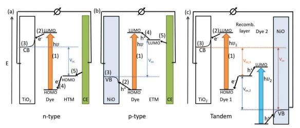
Fig. 28 Charge transfer processes in (a) n-type, (b) p-type and (c) tandem ssDSCs.
