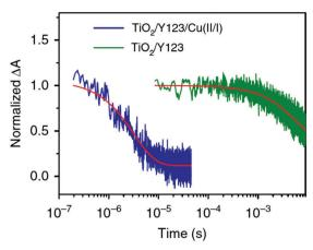
Fig. 9 Transient absorption spectra of Y123-sensitized photoanodes inert (green) and in contact with the solid Cu<sup>II/I</sup>(tmby)<sub>2</sub> hole transport material. Reproduced from ref. 87 with permission from the Nature publishing aroup
