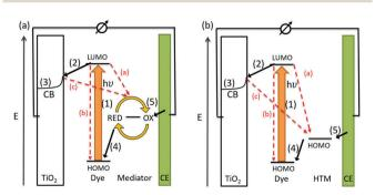
Fig. 2 Schematic drawing of charge transport mechanisms in (a) a liquidjunction DSC and (b) a ssDSC.
