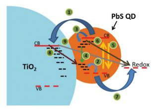
Fig. 19 Schematic illustration of photoinduced charge-transfer processes following absorption of quanta of light by PbS QDs on TiO2. Reprinted from ref. 190 with permission from the American Chemical Society.
