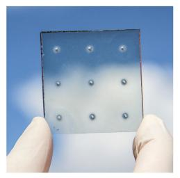
Fig. 27 Electropolymerized poly(3,4-ehtylenedioxythiophene) on an FTO
