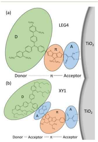
$D-\pi-A/D-A-\pi-A$  structures of the organic dyes (a) **LEG4** and Fig. 16 (b) XY1
