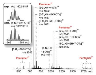
Fig. 5 ESI-Q-TOF-HRMS spectrum of pentameric halogen-bonded capsule 3 (90 μM in CH<sub>2</sub>Cl<sub>2</sub>) with experimental and calculated isotopic
