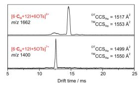
Fig. 3 DT-IM-MS ATDs of ions derived from hexameric halogen-bonded capsule 2. Experimental  $^{\rm DT}CCS_{\rm He}$  and theoretical  $^{\rm TM}CCS_{\rm He}$  values are given.
