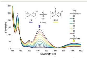
Fig. 2 Variable-temperature UV-vis spectra of [1]<sup>+</sup>[BAr $_1^{F_1}$ ] in THF under 1 atm. N $_2$  ([BAr $_1^{F_1}$ ] counterions omitted). Thermodynamics of N $_2$  binding:  $\Delta H^\circ = -13.1(1)$  kcal mol $^{-1}$ ,  $\Delta S^\circ = -27.6(1)$  cal K $^{-1}$  mol $^{-1}$ ;  $K_{298} = 4.1(3) \times 10^{-3}$  M $^{-1}$ .
