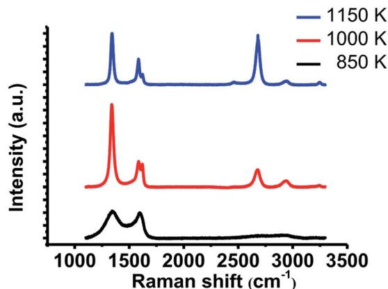
Fig. 3 Raman spectra of the grown films after the transfer onto SiO<sub>2</sub>/Si substrate. All spectra were normalized to the intensity of G band.
