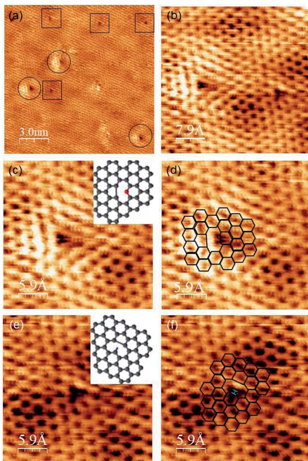
**Fig. 5** (a) and (b) STM images of two types of defects in NG grown at 1150 K.  $V_s$ : 10 mV (c) magnified image of left-hand defect in (b), inset: model of the structure. (d) Magnified images with chemical structure. (e) Magnified images of right-hand defect in (b), inset: model of the structure. (f) Magnified image with chemical structure.
