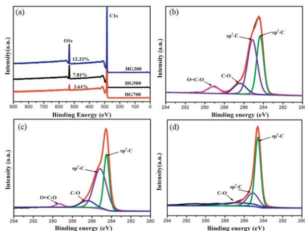
Fig. 5 (a) XPS survey spectra for HG300, HG500 and HG700. (b–d) C1s spectra for HG300, HG500 and HG700.
