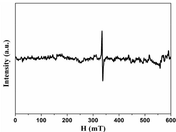
Fig. 8 EPR spectra of HG500 at room temperature.
