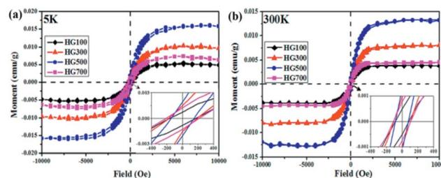
Fig. 6  $M-H$  curves for HG100, HG300, HG500 and HG700 at 5 K (a) and room temperature (b) after subtracting the high field linear background. The insets are the zoom-in part of the hysteresis loops which reveals the soft magnetic character of the hydrogenated graphite.
