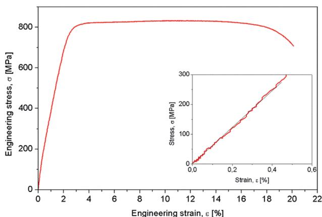
Fig. 3 Strain–stress curve of Ti-31.7Nb-6.21Zr-1.4Fe-0.16O (% wt) Gum-type alloy.
