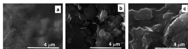
Fig. 6 SEM micrographs of alloy functionalized with SS (a), GNP (b) and GNP-SS (c) by MAPLE (266 nm, 600 mJ cm<sup>-2</sup>). Scale bar: 4 μm.
