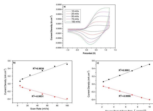
Fig. 3 (a) Cyclic voltammogram of PEDOT nanofibers in  $0.1\text{ M} \text{NBu}_4\text{PF}_6/\text{ACN}$  at various scan rates, and plots of the anodic and cathodic peak current densities vs. (b) the scan rate, (c) the square root of the scan rate.
