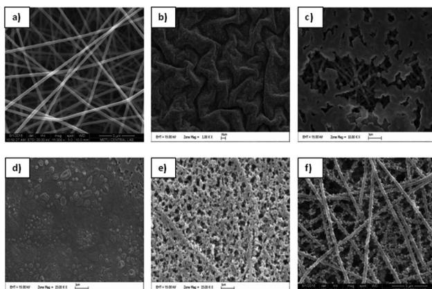
Fig. 1 SEM images of PAN nanofibers (a) and PEDOT nanofibers that were achieved after polymerization periods of (b) 24 h, (c) 3 h, (d) 10 min, (e) 5 min, and (f) 15 min.
