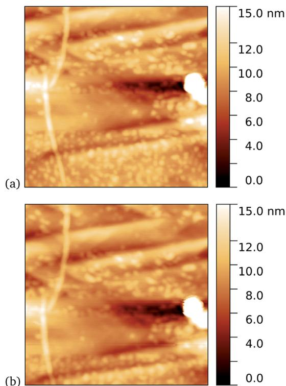
Fig. 9 Results of incubation of 5 nM concentrations of *cyt b<sub>562</sub>-azF* molecules with graphene for 10 minutes with UV illumination, then rinsed for 15 minutes. AFM images of 0.59  $\mu\text{m}$  squares show the proteins are robust to multiple scans. (a) 1st scan of area, (b) 10th scan. The heights of the proteins are around 2 nm.
