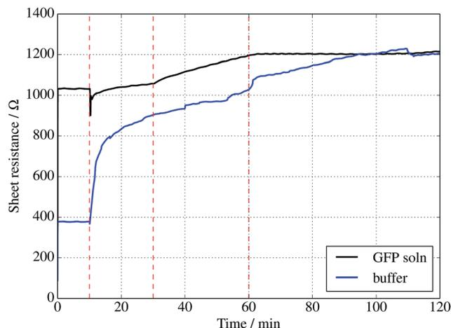
Fig. 4 Sheet resistance of graphene measured in the presence of a  $1 \mu\text{M}$  solution of sfGFP (black curve) solution or buffer solution alone (blue curve). In each case, a droplet was placed onto the centre of a  $1 \text{ cm}^2$  piece of graphene at 10 min, followed by illumination with a 305 nm UV diode between 30 and 60 min only.
