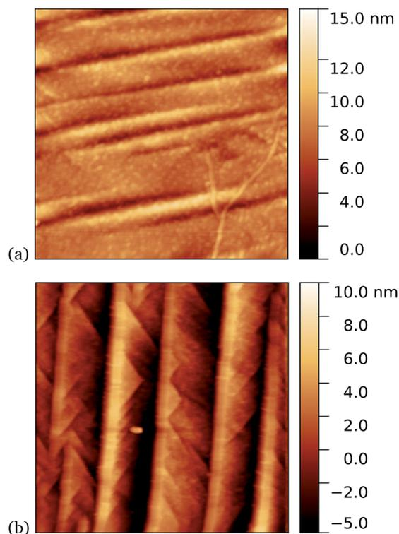
Fig. 8 Results of incubation of 5 nM concentrations of Cyt *b<sub>562</sub>*-azF molecules with graphene for 10 minutes (a) with UV illumination and (b) in the dark, followed by a 5 minute rinse. AFM images of 1 μm square show regions of high coverage for UV but generally much less for the dark.
