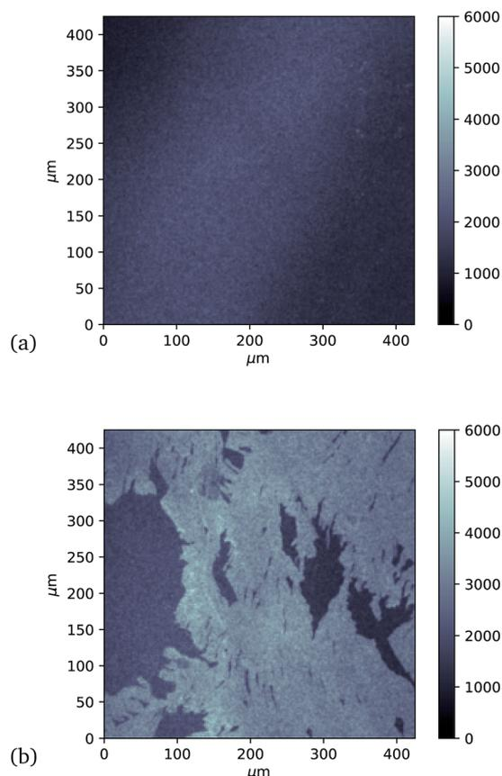
Fig. 5 Approximately  $400 \mu\text{m}$  square confocal microscopy images to compare fluorescence from separate single-layer graphene on silicon samples incubated with GFP204-azF molecules ( $10 \text{ nM}$ ) (a) in the dark and (b) with 10 minute UV exposure, each followed by thorough rinsing with deionised water for one minute. (The vertical intensity scale is arbitrary and the same for each sample.) Images taken using a Zeiss LSM880 confocal laser scanning microscope.
