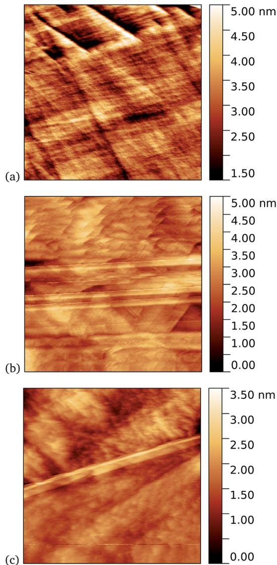
Fig. 10 STM images. (a) A 1.1  $\mu\text{m}$  square image of pristine graphene. After incubation of 10 nM concentration of *cyt b<sub>562</sub>-azF* molecules with graphene for 10 minutes (b) in dark, 0.9  $\mu\text{m}$  square and (c) with UV illumination, 0.4  $\mu\text{m}$  square.
