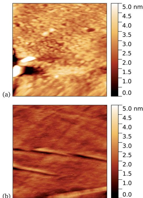
Fig. 6 Results of incubation of  $10 \text{ nM}$  concentrations of TEM105-azF molecules with graphene for 10 minutes (a) with UV illumination,  $0.6 \mu\text{m}$  AFM image and (b) in the dark, followed by a 1 minute rinse,  $1 \mu\text{m}$  AFM image. Regions of high coverage are found for UV but not for the dark.
