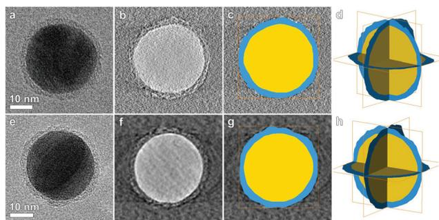
**Fig. 3** (a, e) BF-TEM projection at 0° for, respectively, Ag-L4 and Ag-L8. (b, f) Slices through the reconstructed 3D volumes obtained by weighted back projection and (c, g) superimposed segmentation. Figures (d, h) show the result of the 3D segmentation. The polymer shell (blue) encapsulates the complete particle (yellow). A 3D visualization is shown in the ESI.†
