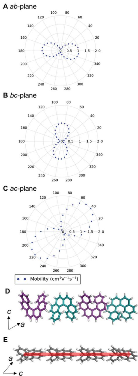
**Fig. 7** Angular-dependent hole-mobility for structure **4** in the (a) *ab*-, (b) *bc*- and (c) *ac*-planes; (d) the adjacent heterochiral chain (substructure type IX) with hole-mobility of  $0.01 \text{ cm}^2 \text{ V}^{-1} \text{ s}^{-1}$  (e) the herringbone translational homochiral chain (substructure type X) with hole-mobility of  $2.0 \text{ cm}^2 \text{ V}^{-1} \text{ s}^{-1}$ . The red arrow shows the highest hole-mobility direction for structure **4**.
