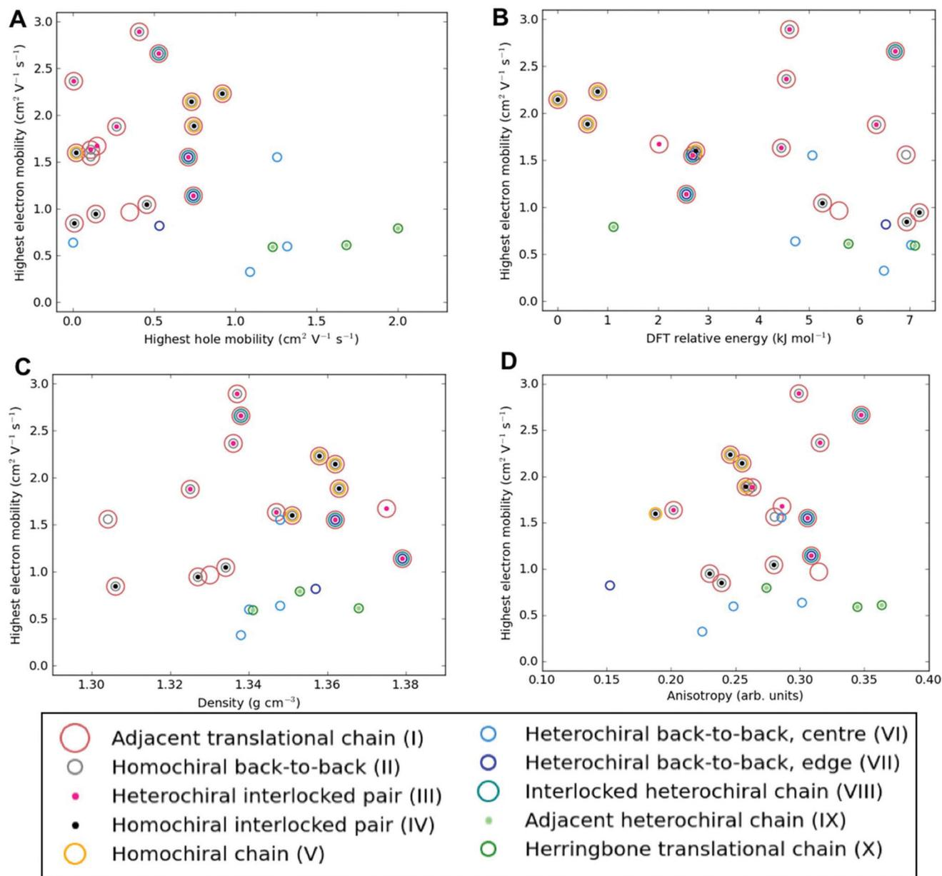
**Fig. 6** Electron-mobility for the energetically low-lying [6]helicene polymorphs compared to (a) hole-mobility, (b) DFT relative energy, (c) density and (d) anisotropy of electron-mobility. The data points are coloured according to the substructure type. The equivalent plots for hole-mobility are in Fig. S10.†
