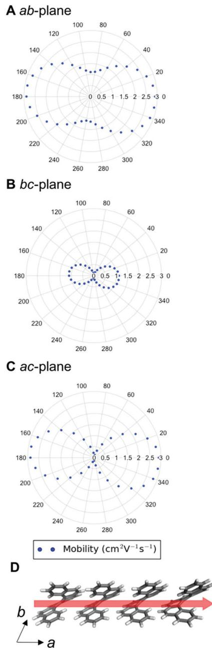
Fig. 8 Angular-dependent electron-mobility for structure **11** in the (a) *ab*-, (b) *bc*- and (c) *ac*-planes; (d) the adjacent translational homochiral chain (substructure type **I**) with electron-mobility of  $2.9 \text{ cm}^2 \text{V}^{-1} \text{s}^{-1}$ . The red arrow shows the highest electron-mobility direction for structure **11**.
