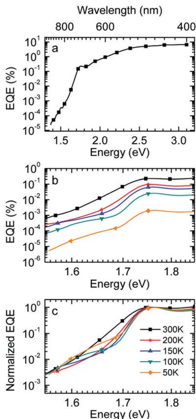
**Fig. 3** (a) External quantum efficiency of MeLPPP:PCBM (1:1) bulk heterojunction devices measured at 300 K over the whole VIS-range down to the sub-bandgap region below 1.7 eV. (b) Temperature dependent EQE for MeLPPP:PCBM (1:1 by weight) blends in the range from room temperature (300 K) to 50 K, shown for the red spectral range. (c) EQE Spectra normalized to the  $S_1$  transition peak of PCBM at about 1.76 eV.
