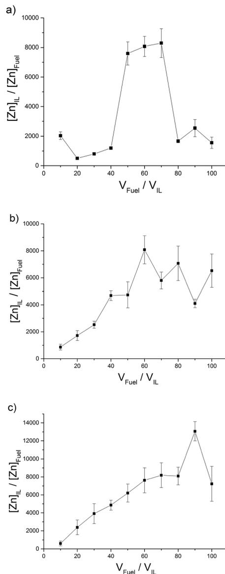
Fig. 2 ILs with high distribution (H) of  $\text{Zn}^{2+}$  into the IL phase; (a)  $[\text{C}_4\text{C}_1\text{im}][\text{Me}_2\text{PO}_4]$  (b)  $[\text{C}_4\text{C}_1\text{im}][\text{S}_2\text{CN}(\text{C}_2\text{H}_5)_2]$  (c)  $[\text{C}_4\text{C}_1\text{im}][\text{OAc}]$ .
