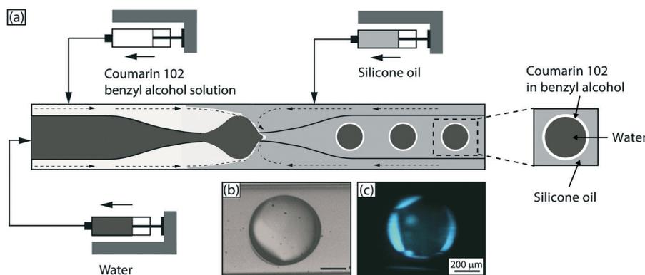
**Fig. 4** (a) A schematic of wrapped laser shell generation. (b) Stereomicroscopic image of  $W/O_1/O_2$  droplets and (c) corresponding stereomicroscopic image of  $W/O_1/O_2$  droplets when excited by a pulsed pump laser beam, highlighting WGM light confinement in the shell.
