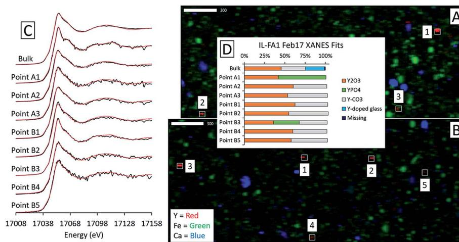
Fig. 8 Synchrotron X-ray spectroscopy analysis of Illinois Basin coal fly ash IL-FA1, including: (A), (B) element maps for two regions of the IL-FA1 thin section collected by  $\mu$ XRF (17 100 eV; scale bars are in  $\mu$ m) showing Y, Fe, and Ca locations, (C) Y K-edge bulk and micro-focus XANES spectra with linear combination fits indicated in red and (D) fit weights. The fitting region was 17 008 eV to 17 158 eV for two regions of the IL-FA1 thin section.
