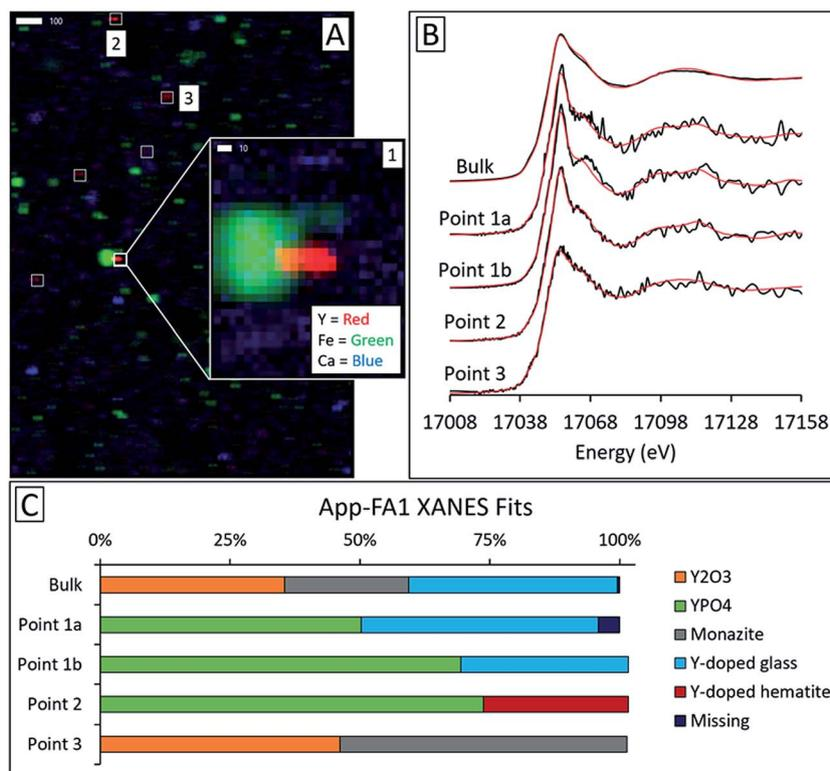
Fig. 6 Synchrotron X-ray spectroscopy analysis of Appalachian silo ash App-FA1, including: (A) element maps collected by  $\mu\text{XRF}$  (17 100 eV; scale bars are in  $\mu\text{m}$ ) showing Y, Fe, and Ca locations, (B) Y K-edge bulk and micro-focus XANES spectra with linear combination fits indicated in red, and (C) fit weights. The fitting region was 17 008 eV to 17 158 eV. Points 1a and 1b were two separate scans of the same yttrium hotspot.
