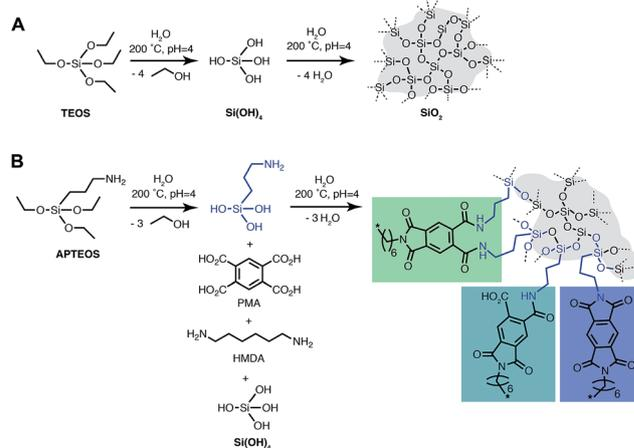
Fig. 4 Reaction equation of SiO<sub>2</sub> and PI6/SiO<sub>2</sub> co-condensation. (A) Hydrothermal hydrolysis and condensation sequence from TEOS to SiO<sub>2</sub>. (B) Co-condensation of PI6 and SiO<sub>2</sub> in the presence of the compatibilizer APTES; possible linkages (1,2-diamide, amic acid; and imide) are shown.
