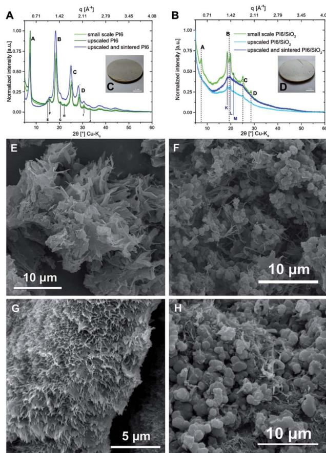
Fig. 7 PI6 and PI6/SiO<sub>2</sub> upscaling and sintering. (A) and (B) Comparison of the diffractograms of small scale synthesis, upscaled synthesis and material after sintering (PI6: (A) PI6/SiO<sub>2</sub>: (B)). (C) and (D) Photographs of the PI6 (C), and the PI6/SiO<sub>2</sub> pellet from sintering. (E)–(H) SEM images of upscaled PI6 before (E) and after (G) sintering, and of upscaled PI6/SiO<sub>2</sub> before (F) and after (H) sintering.
