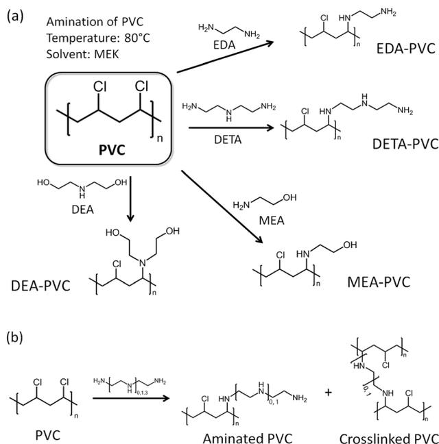
**Fig. 1** (a) Possible amination route of PVC with the selected amines; EDA = ethylenediamine, DETA = diethylenetriamine, MEA = monoethanolamine, DEA = diethanolamine and MEK = methyl ethyl ketone, and (b) a possible crosslinking mechanism for two products functionalized by diamine precursors.
