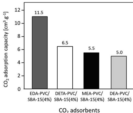
Fig. 7 CO<sub>2</sub> adsorption capacity of APVC/SBA-15 (4%) composites depending on the nature of the aminating reagent.
