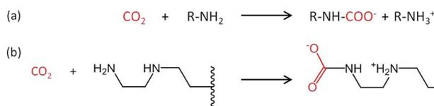
Fig. 8 Proposed reaction schematic for CO<sub>2</sub> chemisorption on a generic amine (a) and supported ethylenediamine (EDA) with carbamate formation in anhydrous condition (b).<sup>31</sup>
