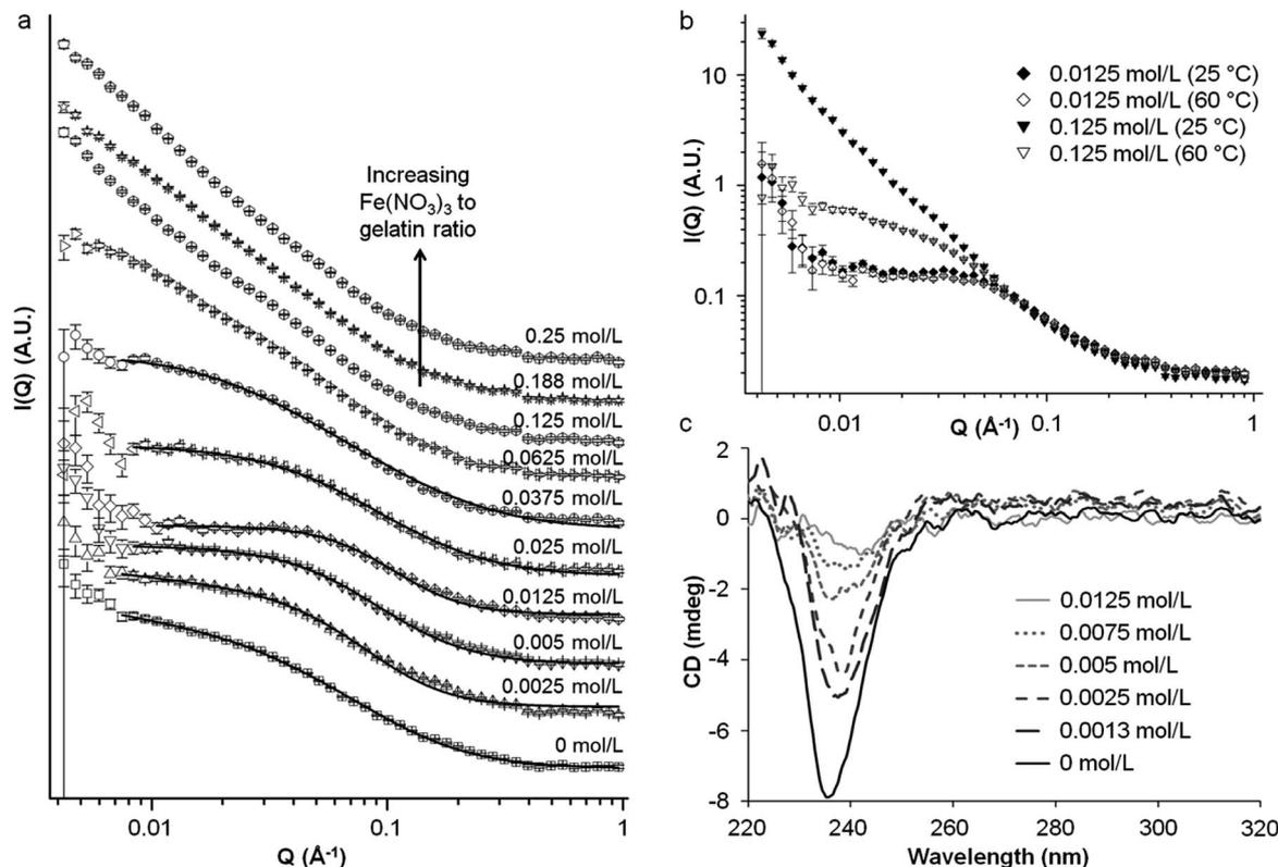
Fig. 5 (a) SANS data for gelatin (5% w/v in water) with various concentrations of  $\text{Fe}(\text{NO}_3)_3$  at  $25 \text{ }^\circ\text{C}$  and (b) SANS data for two Fe : gelatin ratios at  $25 \text{ }^\circ\text{C}$  and  $60 \text{ }^\circ\text{C}$ . (c) Circular dichroism data for a series of gelatin (1% w/v in water) samples with various concentrations of  $\text{Fe}(\text{NO}_3)_3$  at  $25 \text{ }^\circ\text{C}$ . Statistical error bars are smaller than the plotting symbols.
