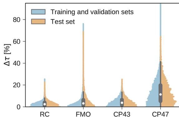
Fig. 3 Normalized distributions of the average relative absolute error of predicted exciton transfer times and exciton transfer times computed with HEOM. The left (blue) side of the plots illustrate the distributions of average relative absolute errors for predictions on the training and the validation set, while the right (orange) side of the plots illustrates the errors for predictions on the test set.
