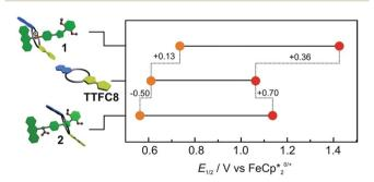
Fig. 5 Correlation diagram of half-wave potentials for charged [2] rotaxane 1, macrocycle TTFC8 and neutral, acetylated [2]rotaxane 2. Half-wave potentials were determined by cyclic voltammetry measurements in  $CH_2Cl_2$  against  $Fe(Cp*)_2^{0/+}$  with a 1 mM analyte concentration at a scan rate of 100 mV s<sup>-1</sup> with tetrabutylammonium BArF<sub>24</sub> (0.1 M) as the electrolyte.
