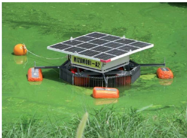
Fig. 22 Photograph of a self-propelled in-liquid plasma apparatus floating over a dam to destroy the harmful Microcystis aeruginosa . Reproduced from ref. 251. Copyright Kumamoto University, Japan.
