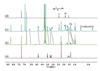
Fig. 5 Partial  $^1$ H NMR spectra (400 MHz, CDCl<sub>3</sub>, 298 K) of (a) 1; (b) 3 (10 mM) with 2 equiv. of 1 and 2; (c) after addition of 2.5 equiv. of adiponitrile to (b); and (d) adiponitrile. The asterisk symbols indicate complexed protons from  $2 \supset$  adiponitrile.
