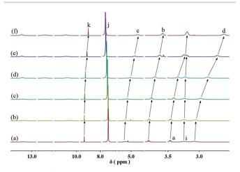
Fig. 2 Partial  $^{1}$ H NMR spectra (400 MHz, CDCl<sub>3</sub>, 298 K) of the mixed solution of 1, 2, and 3 in a 2 : 2 : 1 molar ratio at different concentrations of 3: (a) 3; (b) 5; (c) 10; (d) 20; (e) 40; and (f) 50 mM.
