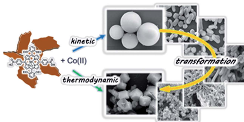
Fig. 5 A series of narrowly dispersed nano- and micro-sized CPs prepared from a Mn(III)-Pp metalloligand acid and Co(OAc) 2 , which morphologies diversified from amorphous spheres to crystalline cubes by varying reaction periods. [Reproduced from ref. 85 with permission from The Royal Society of Chemistry.]
