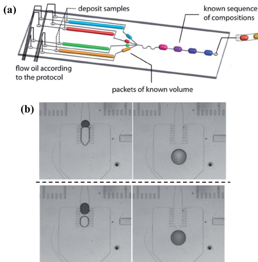
Fig. 9 Droplet coalescence systems to obtain molecular gradients. (a) Simultaneously generation of individual droplets controlled by external electrovalves (reproduced from ref. 172 with permission from the Royal Society of Chemistry). (b) Pillars used to realize fusion without the demand for the synchronization, while the upper line and lower line show passive coalescence with different volume ratios, respectively (reproduced from ref. 174 with permission from Springer).
