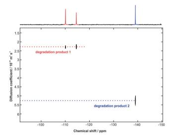
Fig. 5 470 MHz <sup>19</sup>F DOSY spectrum, with the least attenuated 1D spectrum shown at the top, acquired immediately following the <sup>1</sup>H DOSY experiment of Fig. 4
