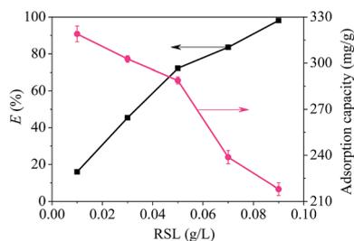
Fig. 9 Effects of adsorbent dosage on the removal of mercury(II). Condition:  $T = 300$  K,  $C_0 = 20$  mg L<sup>-1</sup>, pH = 7.0 ± 0.1.
