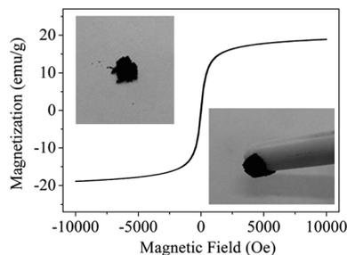
Fig. 6 Magnetization curve of the magnetic PPy-GO.
