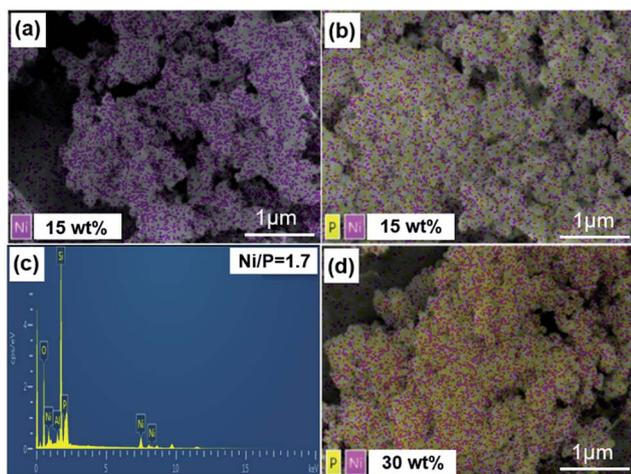
Fig. 2 The SEM and EDS mapping images of different catalysts (red dot refer to nickel atom, and yellow dot refer to phosphorus atom). (a) 15 wt% Ni-Al-M, (b) 15 wt% Ni<sub>x</sub>P-Al-M-(1.25), (c) 15 wt% Ni<sub>x</sub>P-Al-M-(1.25), and (d) 30 wt% Ni<sub>x</sub>P-Al-M-(1.25).
