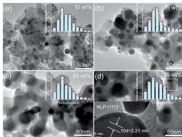
Fig. 3 The TEM images of Ni<sub>x</sub>P-Al-M catalysts synthesized at 650 °C from Ni(NO<sub>3</sub>)<sub>2</sub>·6H<sub>2</sub>O and NH<sub>4</sub>H<sub>2</sub>PO<sub>4</sub> precursors with a mole ratio of Ni/P = 1.25, and with different loadings: (a) 10 wt%, (b) 15 wt%, (c) 20 wt%, (d) 30 wt%. Inset is the corresponding particle size distribution histogram.
