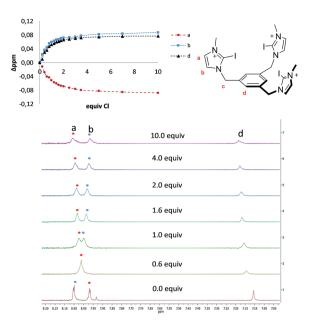
Fig. 1 Representative region of the  $^{1}$ H NMR (500 MHz) spectra of the titration of [1-I](PF<sub>6</sub>) (2 mM) with tetrabutylammonium chloride (100 mM) in DMSO- $d_6$ . The plot represents the binding isotherms.
