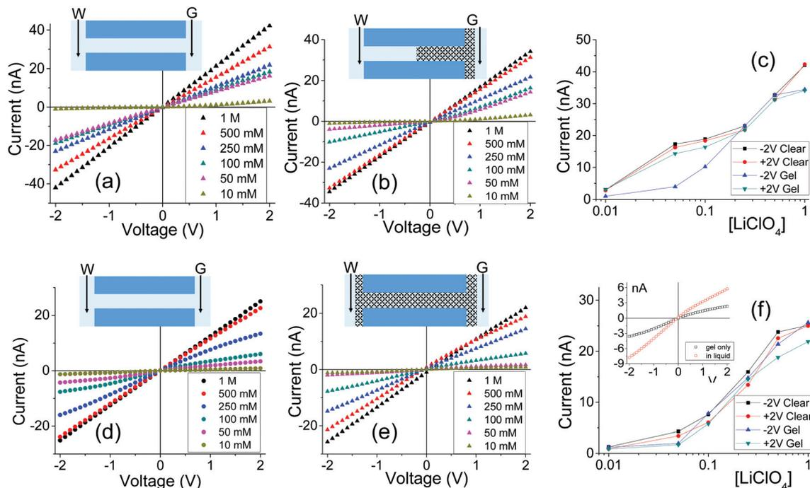
**Fig. 2** (a–c) Ion current through a 790 nm in diameter cylindrical pore subjected to one-sided casting of undoped PMMA. (d–f) Experiments with a 640 nm pore after it had been filled with PMMA gel doped with 100 mM LiClO<sub>4</sub> (drop-casting had been performed on both sides of the membrane). Insets show state of the pore during the *I*–*V* scan. Inset on 3f shows *I*–*V* measurements of gel-only case and the immersed sample (100 mM LiClO<sub>4</sub>/PC).
