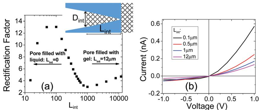
Fig. 7 (a) Scheme of a nanopore system subjected to numerical modeling. The pore considered had opening diameters of 25 nm and 500 nm; the pore length was 12  $\mu\text{m}$ . (b) Modeled  $I$ - $V$  curves for four different values of  $L_{\text{int}}$ .
