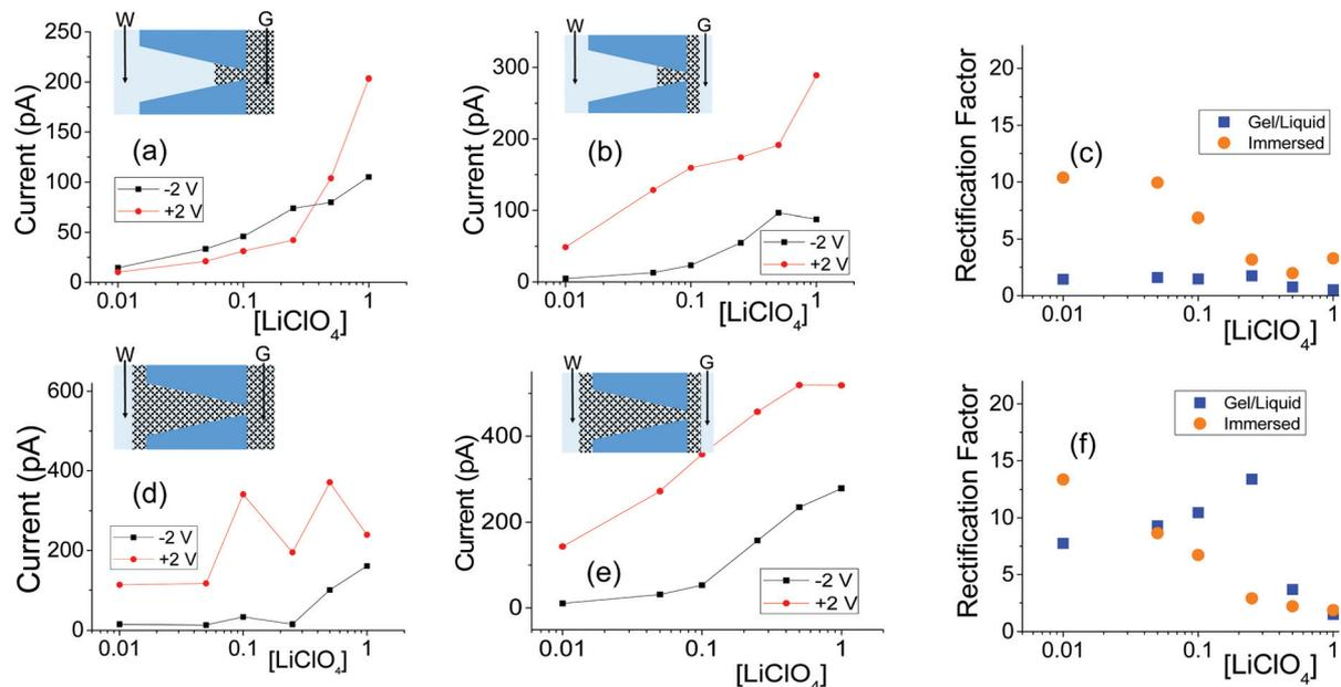
**Fig. 6** (a, b) Recordings with a single conical nanopore with opening diameters of 515 nm (base) and 16 nm (tip); this pore was subjected to one-sided drop cast of PMMA gel doped with 100 mM  $\text{LiClO}_4$ . (d, e) Measurements from another conical nanopore (1080 nm (base) and 18 nm (tip)), filled with PMMA gel. The base side was initially exposed to liquid electrolyte for the GLI test. Another set of data obtained with independently prepared pores is shown in Fig. S7.†
