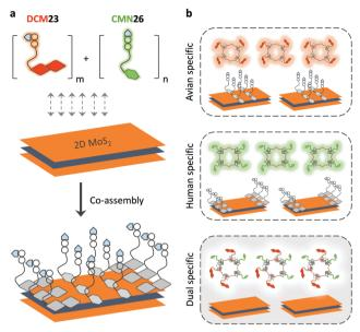
Fig. 5 Schematic illustration of (a) the co-assembly of two sialyl glycan probes tagged with different fluorophores to 2D MoS<sub>2</sub> and (b) the use of a multiplexed system for the detection of influenza viruses with single or dual glycan specificities, where DCM23 and CMN26 are dicyanomethylene 4H-pyrantagged Neu5Acα2,3Gal-β1,4Glc and coumarin-tagged Neu5Acα2,6Galβ1,4Glc probes, respectively. Reprinted with permission from ref. 21. Copyright: The Royal Society of Chemistry.
