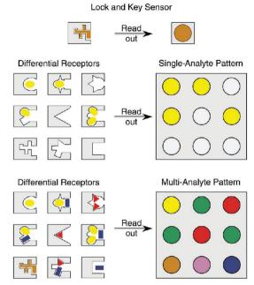
Fig. 13 Schematic illustration of the concept of differential sensing (array sensing) for single and multiple analytes. Reproduced with permission from ref. 45. Copyright: John Wiley & Sons.
