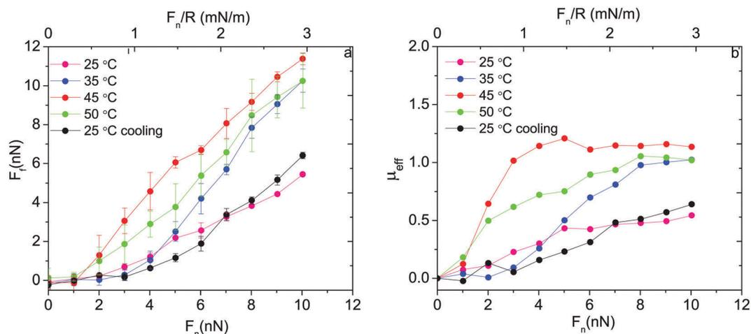
Fig. 3 (a) Friction force and (b) effective friction coefficient,  $\mu_{\text{eff}} = F_f/F_n$ , as a function of applied normal load between silica surfaces carrying a preadsorbed layer of PIPOZ<sub>60</sub>-*b*-PAMPTMA<sub>17</sub> measured at different temperatures. Reproduced with permission from ref. 16. Copyright, 2017 American Chemical Society.
