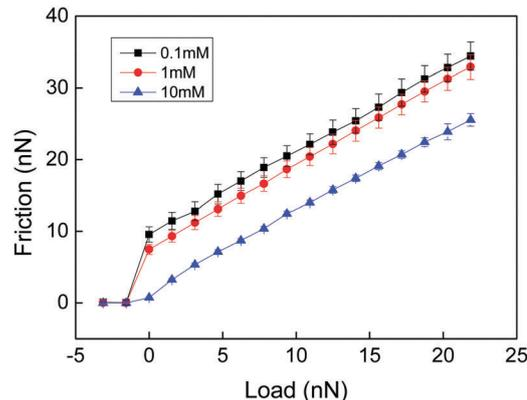
Fig. 2 Friction force vs. load measured between a cross-linked chitosan hydrogel and a silica probe across NaCl solutions of different ionic strengths at pH 5.7. There is no hysteresis between the loading and unloading curves. The error bar is calculated from 10 consecutive measurements. The shear velocity was  $20 \mu\text{m s}^{-1}$ . Reproduced with permission from ref. 29. © 2017 Elsevier Inc.
