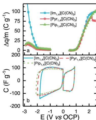
Fig. 4 Electrochemical stability window determination. (a) difference between  $q_{\text{charge}}$  and  $q_{\text{discharge}}$ . (b) CV at determined limit voltage for positive and negative sweep for the ILs [Im<sub>1,4</sub>][C(CN)<sub>3</sub>] (blue), [Pyr<sub>1,4</sub>][C(CN)<sub>3</sub>] (red) and [Pip<sub>1,4</sub>][C(CN)<sub>3</sub>] (green).
