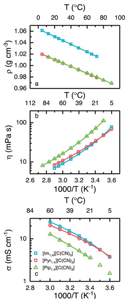
Fig. 3 (a) Density, (b) viscosity and (c) ionic conductivity of the ionic liquids  $[\text{Im}_{1,4}][\text{C}(\text{CN})_3]$  (blue),  $[\text{Pyr}_{1,4}][\text{C}(\text{CN})_3]$  (red) and  $[\text{Pip}_{1,4}][\text{C}(\text{CN})_3]$  (green). Lines in (a) represent density linear fits, and (b) and (c) represent the best VTF fits.
