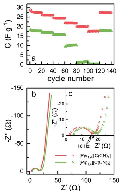
Fig. 6 (a) Specific capacitance obtained from galvanostatic charge-discharge cycling at the different rates 0.5, 1.0, 2.0, 5.0, 7.5, 10 and back to  $0.5 \text{ A g}^{-1}$ . (b) Nyquist plots from EIS measurements and (c) inset showing high frequency semi-circle.
