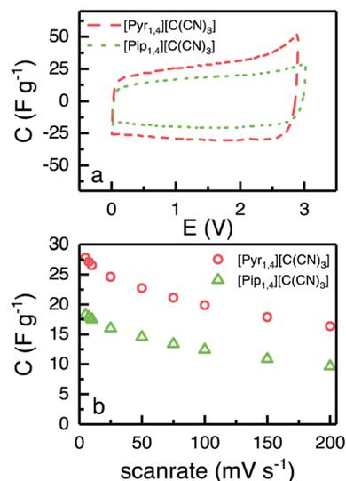
Fig. 5 (a) CVs of EDLC containing  $[\text{Pyr}_{1,4}][\text{C}(\text{CN})_3]$  (red) and  $[\text{Pip}_{1,4}][\text{C}(\text{CN})_3]$  (green) at  $5 \text{ mV s}^{-1}$ , from 0 to 2.9 and 3.0 V, respectively. (b) Calculated capacitance from CVs at different scanrates.
