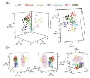
Fig. 4 LDA analyses of  $Ru^{2+}(bpy)_3$  surface mimetic **1–8** array (a) LDA of Ru<sup>2+</sup>(bpy)<sub>3</sub> complex array with eight target proteins achieves clustering of the analytes (each panel represents a different orientation of the data to aid visualization), (b) 80% confidence ellipsoids for the data shown in (a), (conditions as given in Fig. 2).
