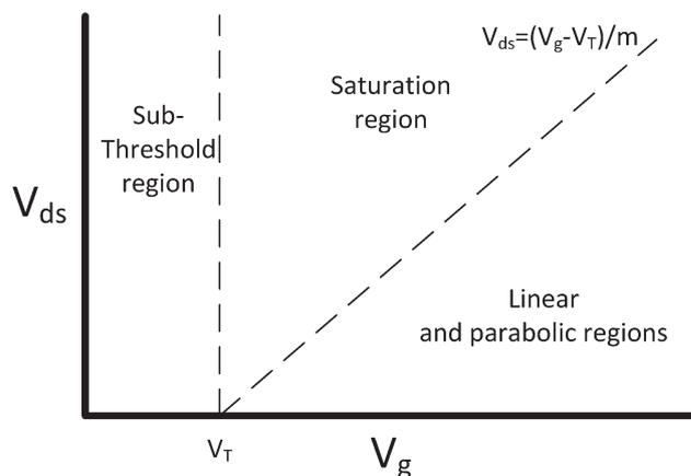
**Fig. 2** FET regions of operation.  $m$  is the body-effect coefficient ( $m \geq 1$ ). Adapted from figure by Taur and Ning (2013).<sup>58</sup>
