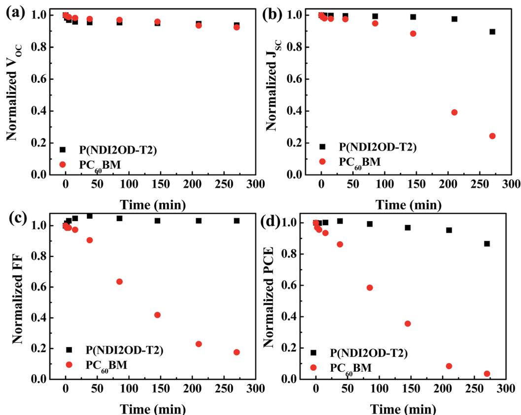
Fig. 4 Variation with time of (a)  $V_{OC}$ , (b)  $J_{SC}$ , (c) FF and (d) PCE of the HPSCs using P(NDI2OD-T2) and PC<sub>60</sub>BM as EELs.
