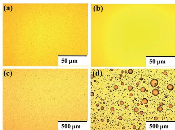
Fig. 5 Optical micrographs of the Al electrode of HPSCs using P(NDI2OD-T2) and PC<sub>60</sub>BM as EELs (a), (b) before (c), and (d) after exposure to ambient conditions.
