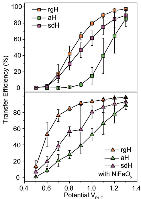
Fig. 4 Charge transfer efficiencies for various hematite photoelectrodes without (top panel) and with (bottom panel) NiFeO<sub>x</sub> decorations at different applied potentials.
