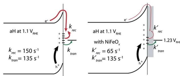
Fig. 8 Surface decorations on hematite improves the overall PEC performance by reducing surface recombination. Compared with bare hematite (left),  $\text{NiFeO}_x$  does not change  $k_{\text{tran}}$  (right). Instead, it reduces the recombination rate constant ( $k_{\text{rec}}$ ) greatly.
