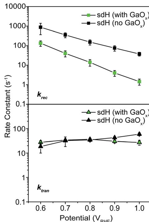
Fig. 5 Rate constants for hematite treated with GaO<sub>x</sub> passivation. Top: recombination; bottom: transfer.
