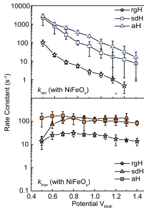
Fig. 3 Rate constants for hematite photoelectrodes with NiFeO<sub>x</sub> surface decorations. Top: recombination rate constants for photoelectrodes by three different preparation methods; bottom: surface charge transfer rate constants for the same photoelectrodes. The error bars are standard deviations between different samples.
