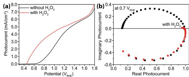
Fig. 6 Characterizations with  $\text{H}_2\text{O}_2$  as hole scavengers. (a) Steady-state current-voltage curves for sdH with (red) and without (black)  $\text{H}_2\text{O}_2$ . (b) IMPS data of sdH with (red) and without (black)  $\text{H}_2\text{O}_2$  at 0.7 V vs. RHE.
