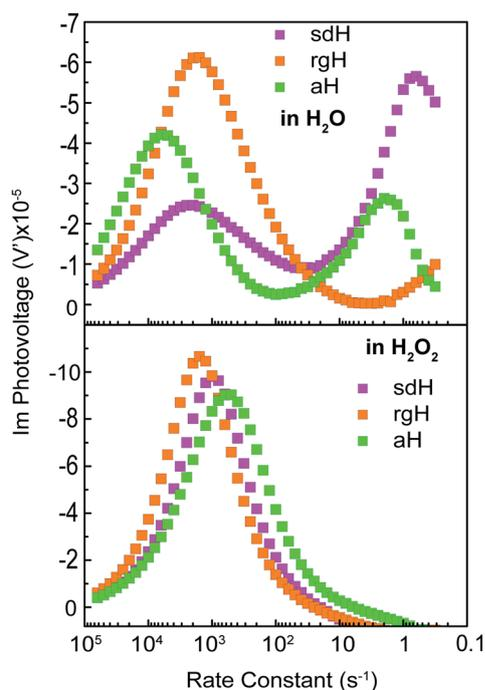
Fig. 7 Intensity modulate photovoltage spectroscopy (IMVS) of various hematite photoelectrodes in  $\text{H}_2\text{O}$  (top) and in  $\text{H}_2\text{O}_2$  (bottom). Data presented as Bode plots, where the Y axis shows the imaginary component of the complex photovoltage, and the X axis shows the rate constants converted from the modulation frequencies.
