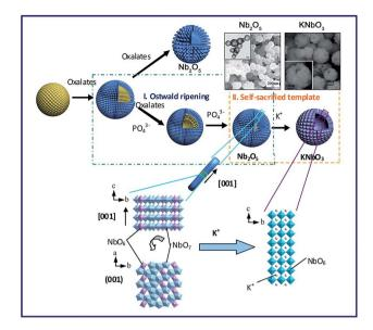
Fig. 4 Formation processes and structure evolution of the  $KNbO_3$  hollow spheres and  $Nb_2O_5$  solid spheres. The insets are the  $Nb_2O_5$  hollow spheres and the  $KNbO_3$  hollow spheres (ref. 31 Copyright 2013, the Royal Society of Chemistry).
