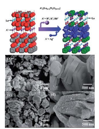
Fig. 8 (Top) Electron density plot of A' $_2$ [La $_{(n-1)}$ Ti $_n$ O $_{(3n+1)}$ ] and Ag $_2$ -La $_2$ Ti $_3$ O $_{10}$ . (a and b) FESEM images of solid-state prepared Rb $_2$ La $_2$ Ti $_3$ O $_{10}$ . (c and d) Silver-exchanged Ag $_2$ La $_2$ Ti $_3$ O $_{10}$  in AgNO $_3$  flux (ref. 30 Copyright 2013, American Chemical Society).
