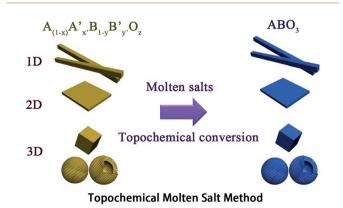
Fig. 1 The schematic illustration of the topochemical molten salt method.
