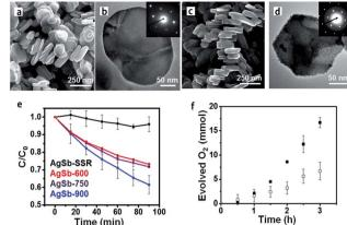
Fig. 7 (a) SEM and (b) TEM images of the NaSbO<sub>3</sub> product obtained from an aerosol-assisted synthesis. (c) SEM and (d) TEM images of the AgSbO<sub>3</sub>, single-crystalline NaSbO<sub>3</sub> plates in molten AgNO<sub>3</sub> were used as the template. (e) Rhodamine B photocatalytic degradation under  $\lambda = 400-500$  nm illumination. (f) Oxygen evolution in the presence of 0.1 M AgNO<sub>3</sub> (ref. 55 Copyright 2015, American Chemical Society).
