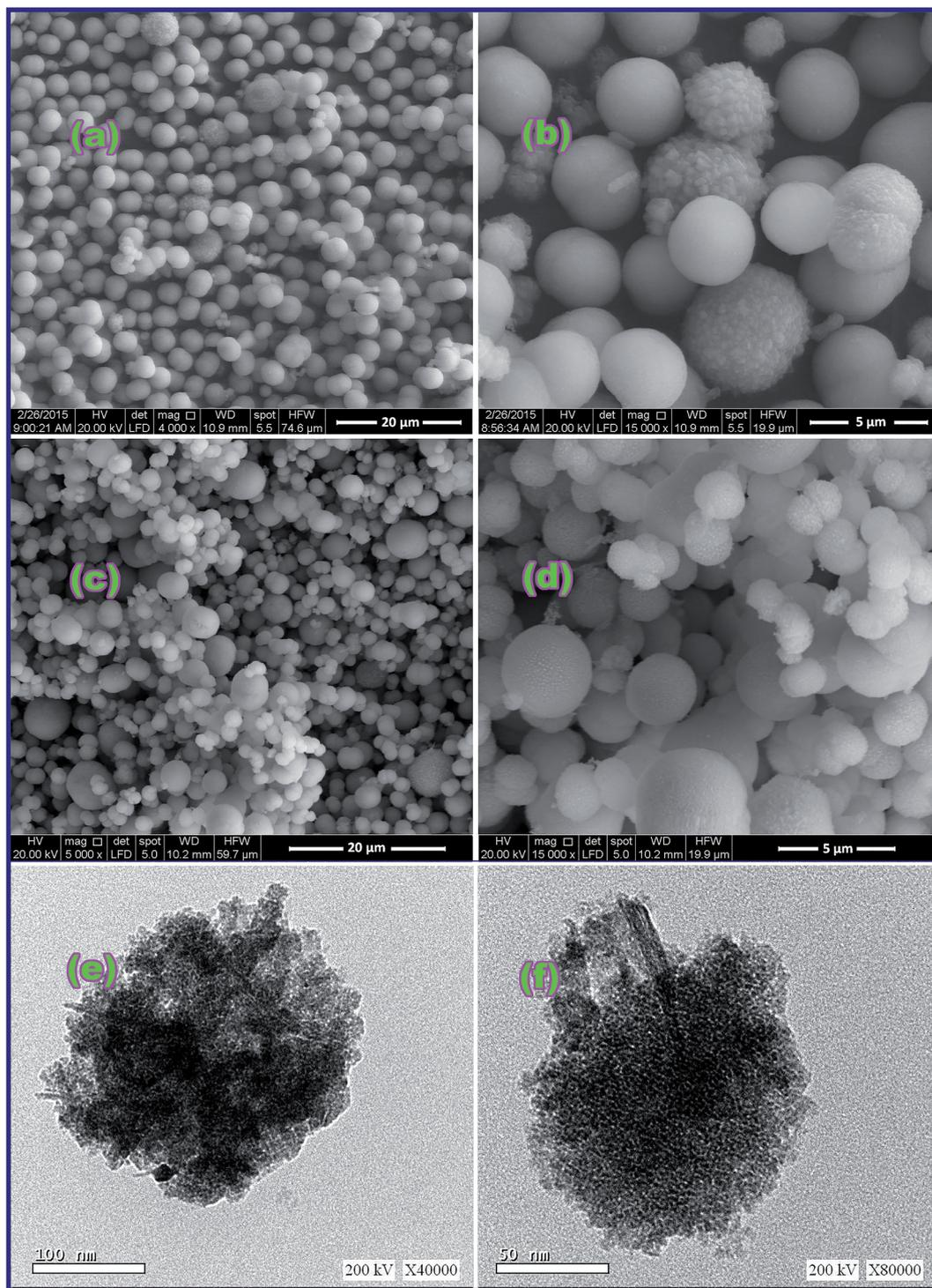
Fig. 4 FE-SEM images of the as-synthesized  $\text{CoCO}_3/\text{FeCO}_3$  nanocomposite (a and b) and  $\text{CoFe}_2\text{O}_4$  product (S46\_600 (c and d)); low and high magnification TEM images of  $\text{CoCO}_3/\text{FeCO}_3$  nanocomposite (e and f), respectively, where (a and c) are low magnification FE-SEM images, while (b and d) are high magnification FE-SEM images.
