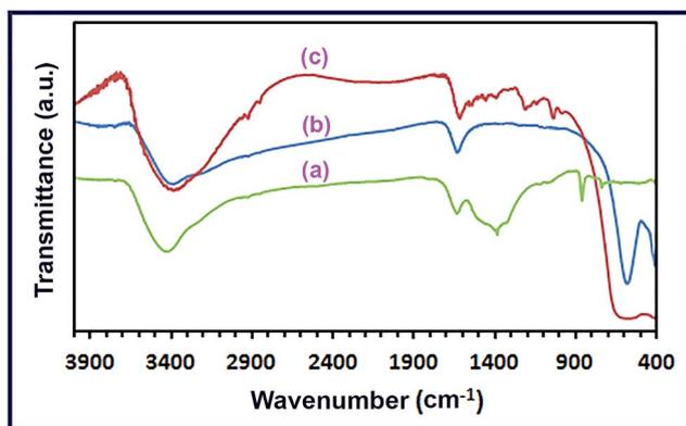
Fig. 5 FT-IR spectra of the as-prepared  $\text{CoCO}_3/\text{FeCO}_3$  nanocomposite (a), spinel  $\text{CoFe}_2\text{O}_4$  (b), and RR195-loaded  $\text{CoFe}_2\text{O}_4$  (c).
