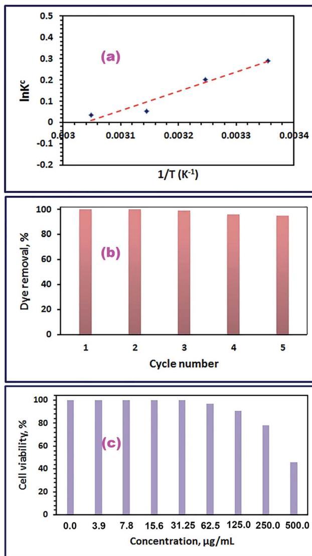
Fig. 13 Plot of  $\ln K_c$  versus  $1/T$  (a), effect of regeneration cycle on the efficiency of  $\text{CoFe}_2\text{O}_4$  adsorbent for RR195 dye removal (b), and cell viability assessment of  $\text{CoFe}_2\text{O}_4$  adsorbent at pH 2 (c).
