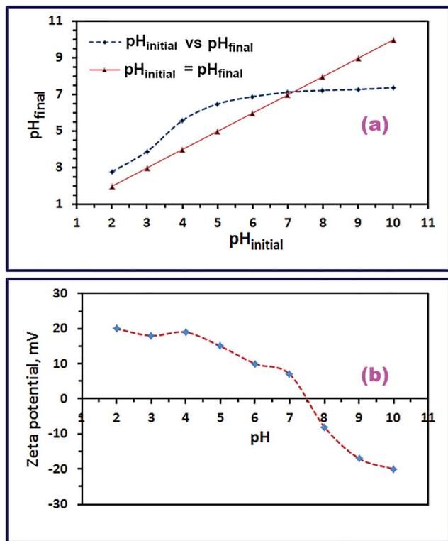
Fig. 9  $\text{pH}_{\text{initial}}$  versus  $\text{pH}_{\text{final}}$  graph for  $\text{pH}_{\text{pzc}}$  calculation for  $\text{CoFe}_2\text{O}_4$  product (a), and zeta potential versus pH graph for IEP estimation for  $\text{CoFe}_2\text{O}_4$  product (b).
