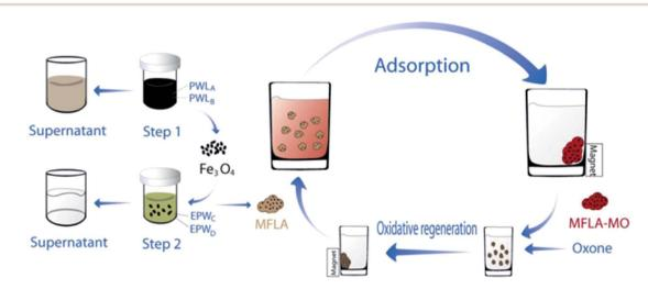
Fig. 8 Synthesis route of MFLA and their application for removal of MO with the help of an external magnetic field (MFLA: magnetic Fe<sub>3</sub>O<sub>4</sub>/Zn-Cr LDH adsorbent, PWL: pickling waste liquor, EPW: electroplating wastewater. Adapted from ref. 70 with Copyright from 2012 Elsevier).
