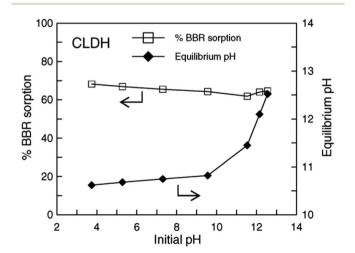
Fig. 6 Effect of initial pH on Brilliant Blue R (BBR) sorption by calcined layered double hydroxides (CLDHs) and on equilibrium pH (adapted from ref. 34 with Copyright from 2005 Elsevier).
