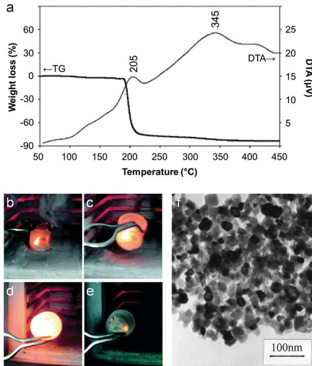
Fig. 4 (a) TGA/DTA trace for a mixture of citrate with barium and iron nitrates showing a sharp combustion at  $\sim 200\text{ }^\circ\text{C}$ . (b–e) Images from a video of a combustion synthesis showing rapid progression of the reaction. (f) TEM image of a sample of a NiCuZn ferrite synthesized from a citrate/nitrate combustion method. Figures modified with permission from ref. 45, 46 and 48 respectively.
