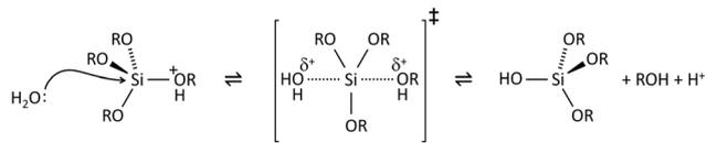
Scheme 1 Acid catalysed hydrolysis of silicon alkoxides.
