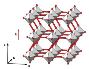
Fig. 5 An antiferroelastic planar shift system characterised by displacements parallel to  $\mathbf{a}$ , correlated with modulation wave-vector  $\mathbf{k} = [0, 0, \frac{1}{2}]$ .
