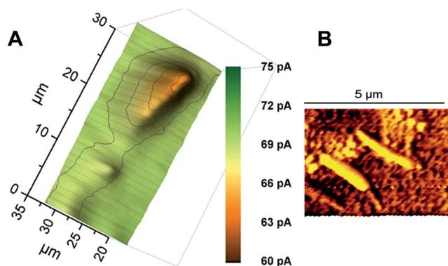
Fig. 2 (A) Negative feedback SECM image of individual AuNWs immobilized on a glass slide. The image was recorded with a  $300 \text{ nm}$  radius Pt probe at a potential of  $0.3 \text{ V}$  and a scan rate of  $5 \mu\text{m s}^{-1}$  in  $1.5 \text{ mM}$  ferrocenemethanol solution. (B) Representative AFM image of AuNWs immobilized on a glass slide.
