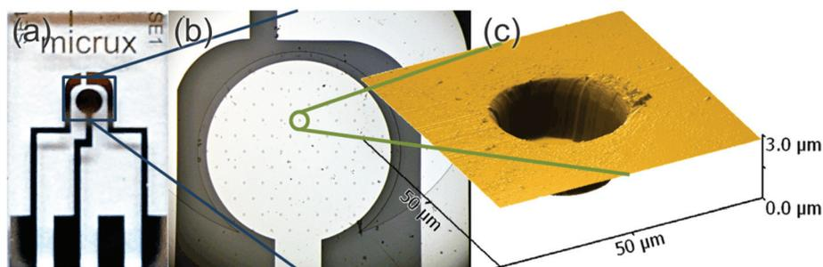
**Fig. 1** (a) Photo of the thin-film microarray electrode, (b) optical microscope image of the platinum working electrode, consisting of a platinum disk electrode ( $\varnothing_{\text{Pt-disk}} = 1 \text{ mm}$ ) covered by a ( $3.0 \pm 0.5 \mu\text{m}$  thick) SU-8 layer and defined by 90 microholes ( $\varnothing_{\mu\text{-hole}} = 10 \mu\text{m}$ , pitch =  $100 \mu\text{m}$ ), (c) atomic force microscopy (AFM) mapping of a working electrode microhole.
