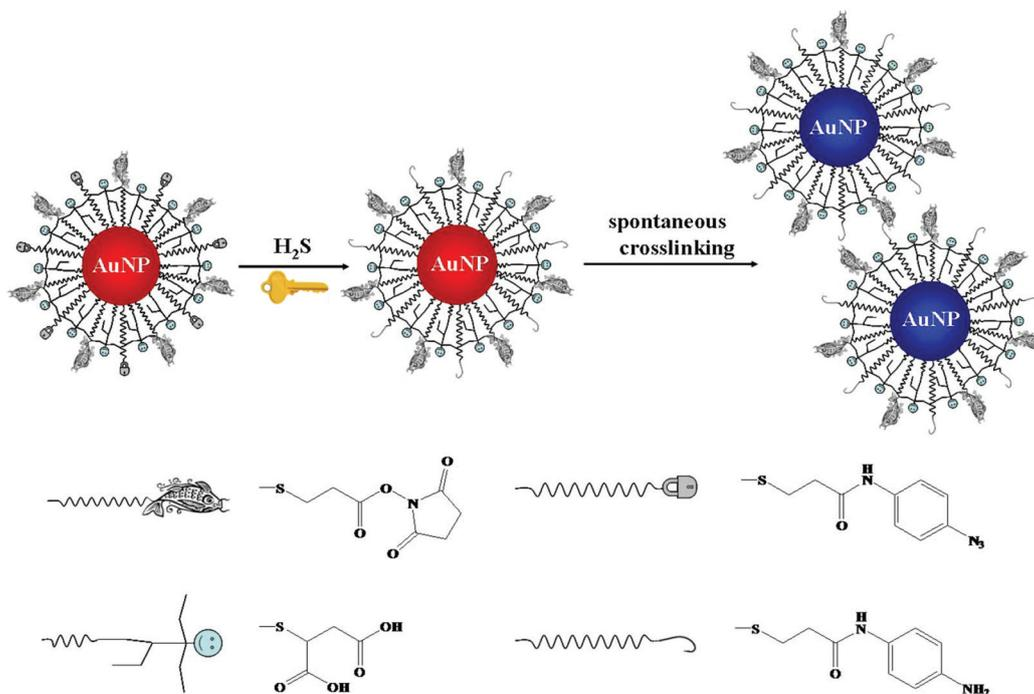
Fig. 3 Schematic representation of the sensing principle of AE-Au NP probes for the detection of H<sub>2</sub>S. Reprinted with permission from ref. 101. Copyright 2015, American Chemical Society.
