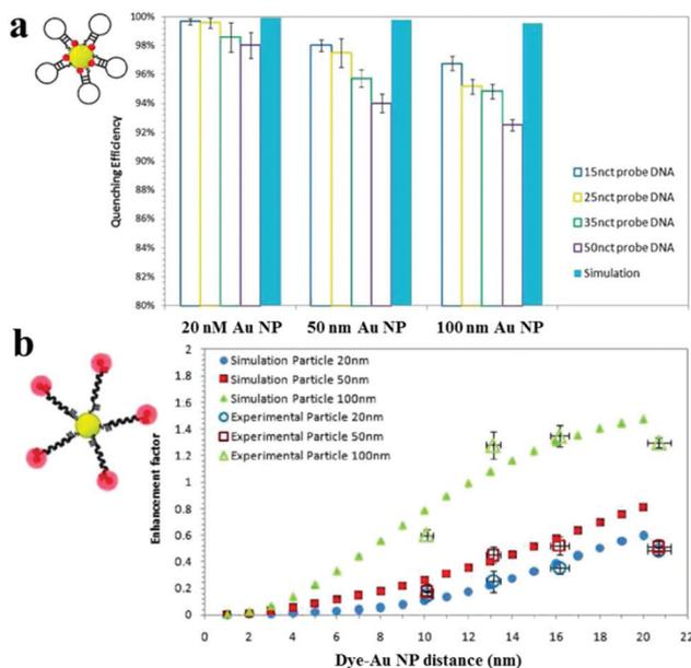
**Fig. 7** Fluorescence quenching and enhancement by Au NP size and dye–Au NP distance. (a) Quenching efficiency as a function of Au NP size and DNA length. (b) Enhancement factor as a function of particle size and dye–Au NP distance. Reprinted with permission from ref. 161. Copyright 2011, American Chemical Society.
