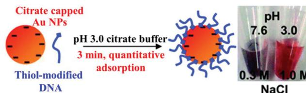
**Fig. 2** Schematic illustration of attaching negatively charged thiolated DNA to negatively charged Au NPs using the low pH assisted method. Reprinted with permission from ref. 48. Copyright 2012, American Chemical Society.
