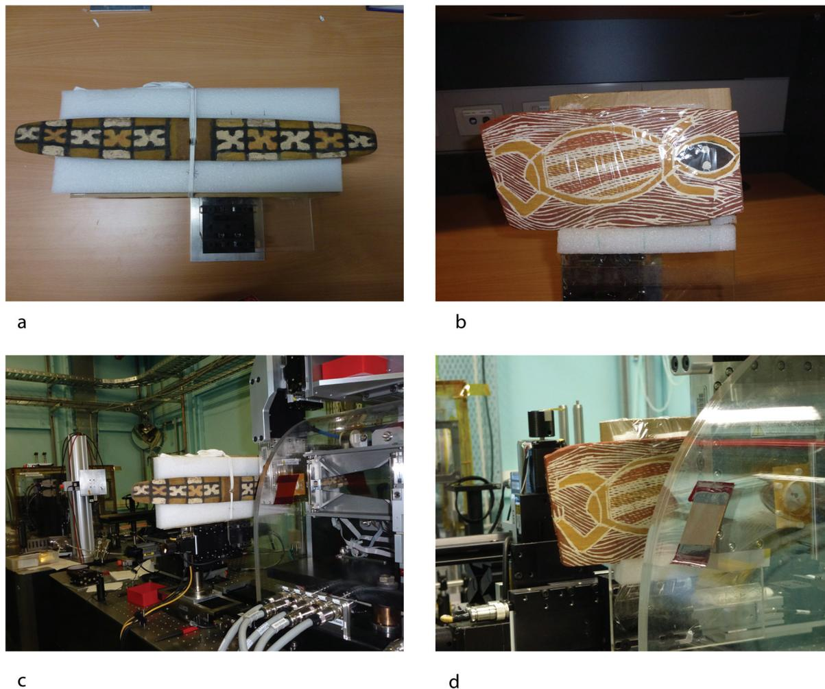
Fig. 1 Objects mounted to the XFM stage (a and b) demonstrating mounting procedures. Objects on the beamline in preparation for XFM analysis (c and d).
