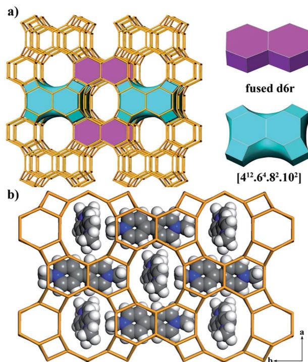
Fig. 1 (a) 3D framework of JU101 showing 10-ring channels along the [001] direction (left). Two characteristic BUs, fused d6r and the  $[4^{12}\cdot 6^4\cdot 8^2\cdot 10^2]$  cavity (right) are highlighted in the framework. (b) Simulated positions of  $MV^{2+}$  cations in the pores viewed along the [001] direction. Colour: C, gray; H, white; N, blue.
